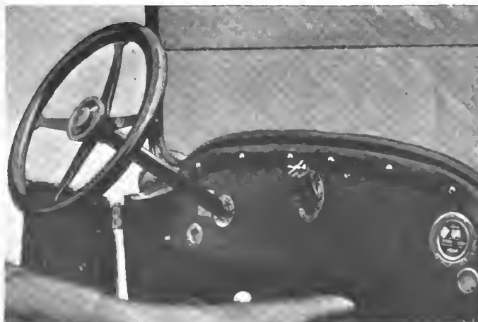
Cowl board and control of new Briscoe. Note unique spark and throttle lever control on wheel
